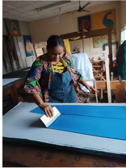
Plate 1d: Coating of the screen
